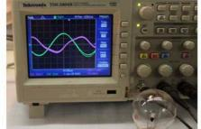
The ReGenX Generator's Load Current Delay can be between 45 and 90 degrees.
